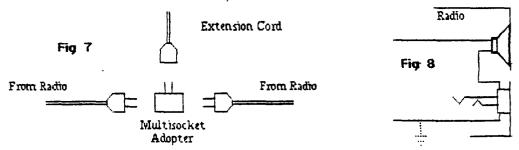
The second and much preferred method, is to install a 1/8" normally closed jack in the speaker circuit of each radio or experimental TR. (Fig 8) Since these jacks are quite small it is usually easy to find some suitable spot in the radio cabinet, near the speaker, where it can be installed. By using a normally closed jack, speaker operation is normal with no plug inserted. Two cables are then made with a corresponding plugs on one end.
