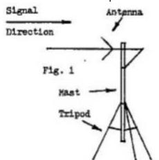
point <u>straight up</u>. (See Fig. 2) Since these antennas are quite\_directional, in the vertical position it would pick up nothing from Earth transmitters, even if there were any nearby. It would, however, be very sensitive to any UHF TV signals that might be beamed down from overhead, even from as far away as the fringes of space.
