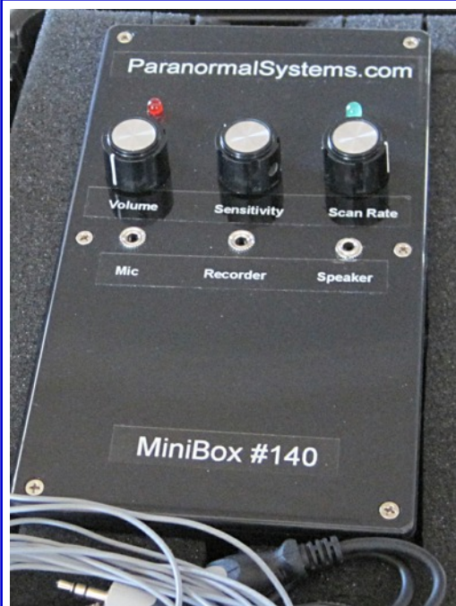
This is a Minibox by Paranormal Systems, Inc. (2007). It is basically a radio equipped with a tuner that automatically sweeps the dial. The sweep is continuous and the rate is variable. See the ATransC endnote.
